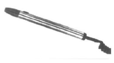
Fig 2-8 A light pen activated with a button switch.
